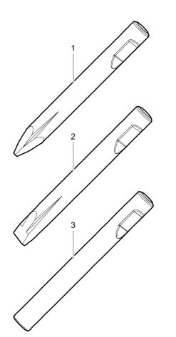
$\varnothing$ =120 mm, L=670 mm, L\_\_=1150 mm, Wt=89.0 kg  $\varnothing$ =4.72 inch, L=26 inch, L\_\_=45.28 inch, Wt=196.2 lb
